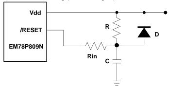
Fig. 35. External Power-Up Reset Circuit
